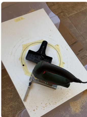
The guide fitted, halfway through the first cut.
